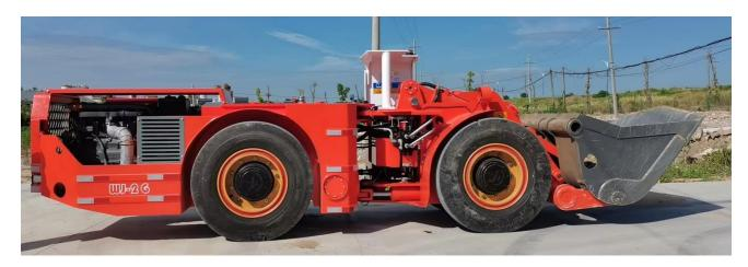
WJ-2G underground wheel loader | Scooptram is central articulated frame underground wheel loader, with S-shape self-balancing structure boom, Cabin set on the rear part of the chassis with FOPs+ROPs open cabin. Wear-resistance shovel blade and side blade from Sweden. NO-SPIN for front axle;
