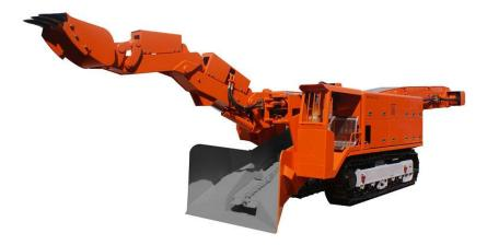
LWLX-60D crawler mucking loader is a continuous excavating, drawing, loading and feeding equipment for material transportation. It is mainly been used in tunnel construction, diversion culvert, cave construction, etc.
