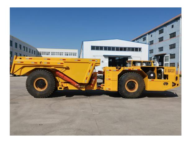
UK-20 Low profile dumper truck is a wheeled transporting equipment designed for underground mining. It works together with LHD underground wheel loader for transporting mine ores and other materials.
