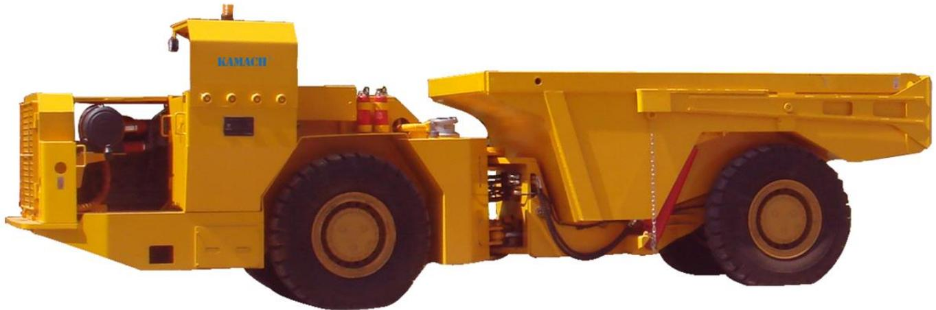
UK-15 Underground MineTruck is used together with WJ-3 or WJ-4 UG production loader. Power supply is emission tire 3 water-cooled diesel engine, to reduce the fuel consumption, and exhaust.
